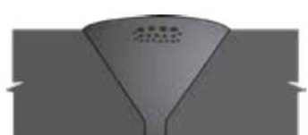
30 Porosity in Single Vee (sub-surface) UT, RT
