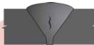
15 Centerline Crack, Single Vee (sub-surface) UT, RT
