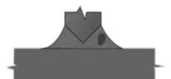
38 Slag Inclusion in Fillet (root area) UT, RT
