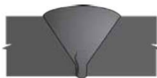
12 Root Crack in Single Vee MT/PT, UT, RT
