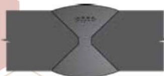
30 Porosity in Double Vee (sub-surface) UT, RT
