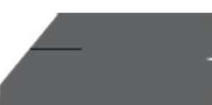
51 Lamination in Weld Prep MT/PT, UT
