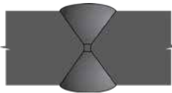
Incomplete Root Penetration in Double Vee, UT, RT
