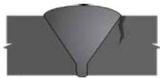
10 Toe Crack in Single Vee MT/PT, UT
