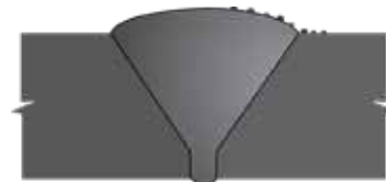
90 Weld Splatter on Single Vee, VT, RT
