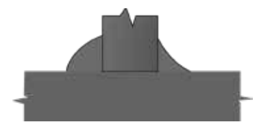
75 Excess Crown in Fillet, VT
