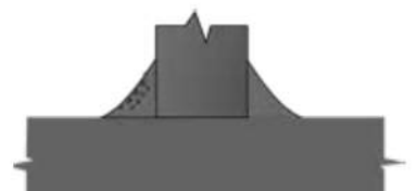
33 Porosity in Fillet (surface breaking) VT, MT/PT
