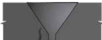
19 Base Metal Crack in Single Vee (bottom HAZ area) MT/PT, UT
