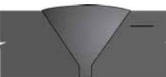
50 Lamination in Single Vee (base metal) UT
