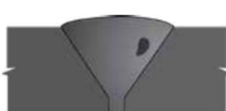
37 Slag Inclusion in Single Vee (weld groove area) UT, RT
