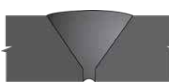
70 Root Concavity in Single Vee VT, RT
