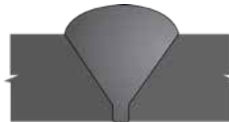
74 Excess Crown in Single Vee, VT
