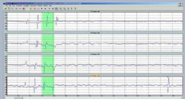
Traces of 1150 m belt length with automatically marked splices (green) and broken cords (triangles).
