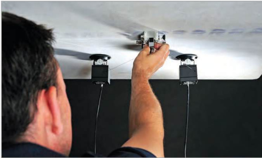
Tracer - Inverted scan inspection
