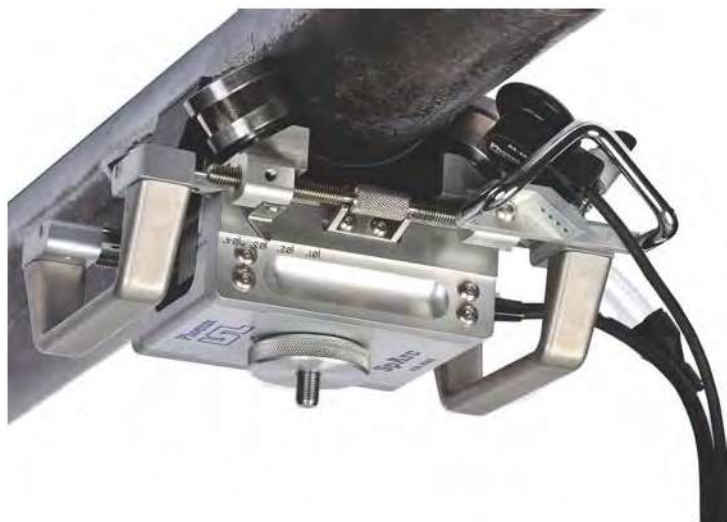
Sp-Arc inspecting the underside of a 3" pipe
