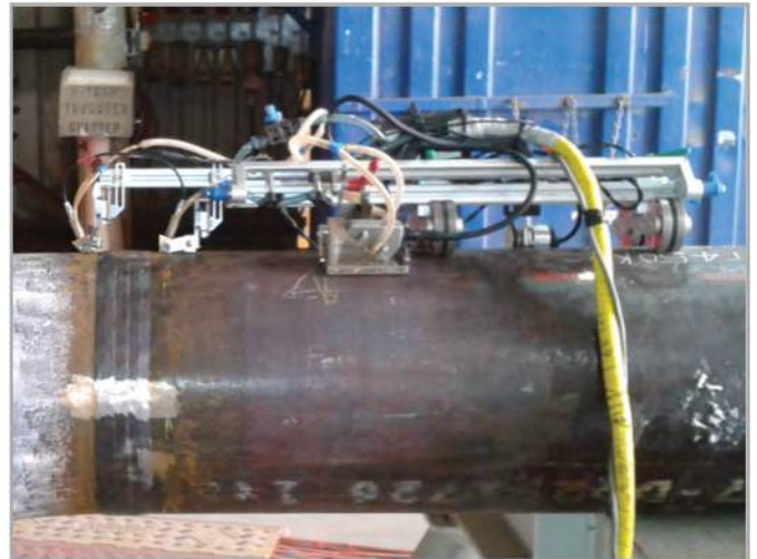
MultiMag with TOFD for pipe elbow inspection
