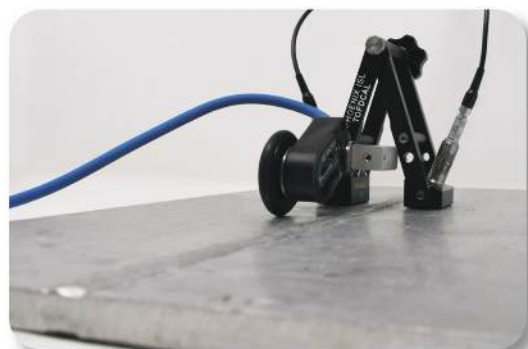
Weld inspection with TOFD Caliper
