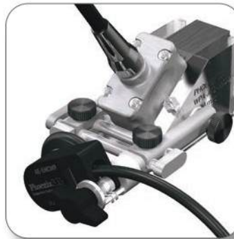
C-Clamp with rear mounted encoder and phased array probe and wedge
