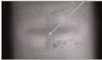
Radiograph showing lack of fusion
