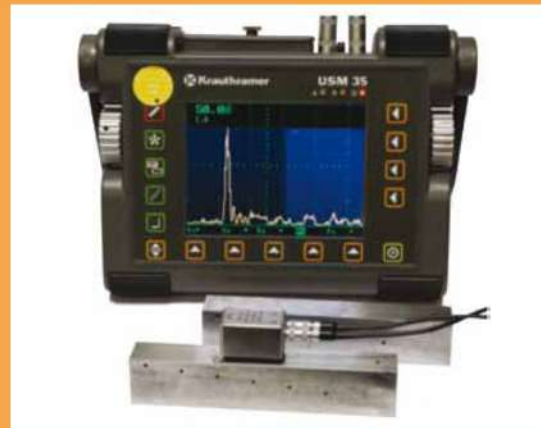
A dual element, longitudinal wave mode probe on austenitic steel
