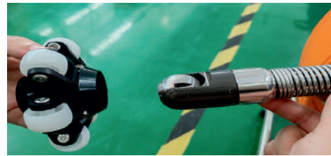
Step2: Install Skid To Camera Head
