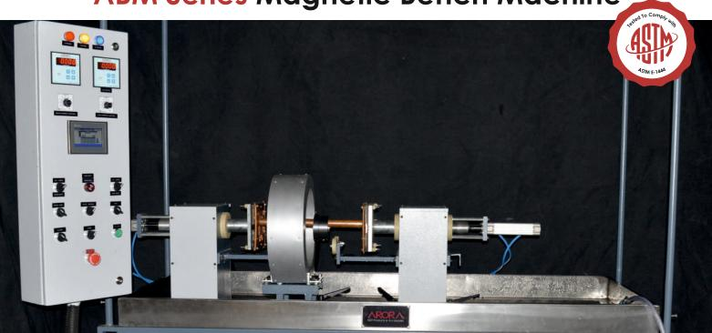
The ABM Series are heavy duty bench machine designed for MPI inspection. The ABM Series magnetic benches are available in Seven configuration and three sizes (Small/Medium/Large) that offers 2000 Amps to 10,000 Amps range of Alternating Current (AC), Half Wave Direct Current (HWDC) or Full Wave Direct Current (FWDC).
