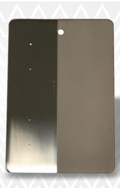
TAM Panel offers a swift and efficient approach to evaluating the ongoing functionality of liquid penetrant inspection systems. It supports various types of penetrants including fluorescent, water wash and non-water wash, hydrophilic and lipophilic, as well as visible ones.
