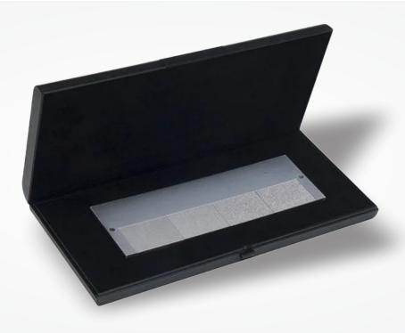
Type 2 Reference Blocks are utilized for the regular evaluation of DPI system performance. These blocks consist of 5 artificial star-shaped defects, ranging from 3.0 to 5.5mm diameters, on one side. Additionally, the 4 adjacent patches on the same side feature different roughnesses of 2.5µm, 5µm, 10µm, and 15µm.
