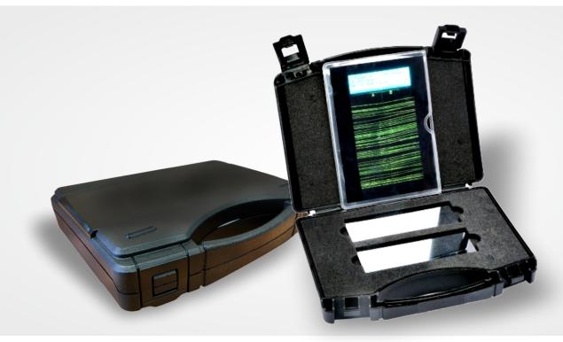
The Ni-Cr Test Panels consist of brass plated with nickel-chrome alloy, deliberately stressed to produce linear cracks in the plating. These cracked test pieces are then divided into two identical panels, allowing for a comparison between materials in use and new, unused materials with identical flaws.
