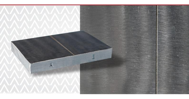
The Aluminum Comparator Block is split into two sections, designed for comparing various penetrants or for comparing fresh penetrant to the one currently in use. Crafted from 2024 Aluminum, this block features a groove dividing the two sides, enabling easy side-by-side comparison of penetrants. It is intended for one-time use only
