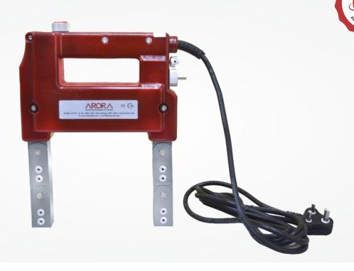
The AY-7D is most versatile magnetic yoke which offers AC and HWDC single phase supply for magnetizing ferromagnetic material. The two outputs (AC or HWDC) are independently adjustable to balance the magnetic field intensity. The AY-7D provides either constant AC or Pulsed HWDC field for finding surface and subsurface defects.
