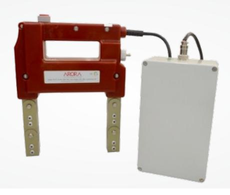
AY-7B is a battery operated portably designed yoke which can be used for magnetic particle inspection in the field and remote locations. The battery provides a 8 hour power enabling it to contour any shape without AC power. The AY-7B provides DC that unable you to find surface and sub surface defects.
