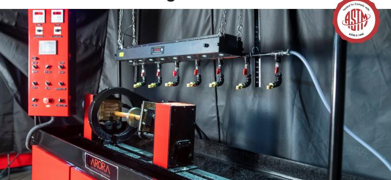
The ABM Series are heavy duty bench machine designed for MPI inspection. The ABM Series magnetic benches are available in Six configuration and three sizes (Small/Medium/Large) that offers 1500 Amps to 6000 Amps range of Alternating Current (AC), Half Wave Direct Current (HWDC) or Full Wave Direct Current (FWDC).
