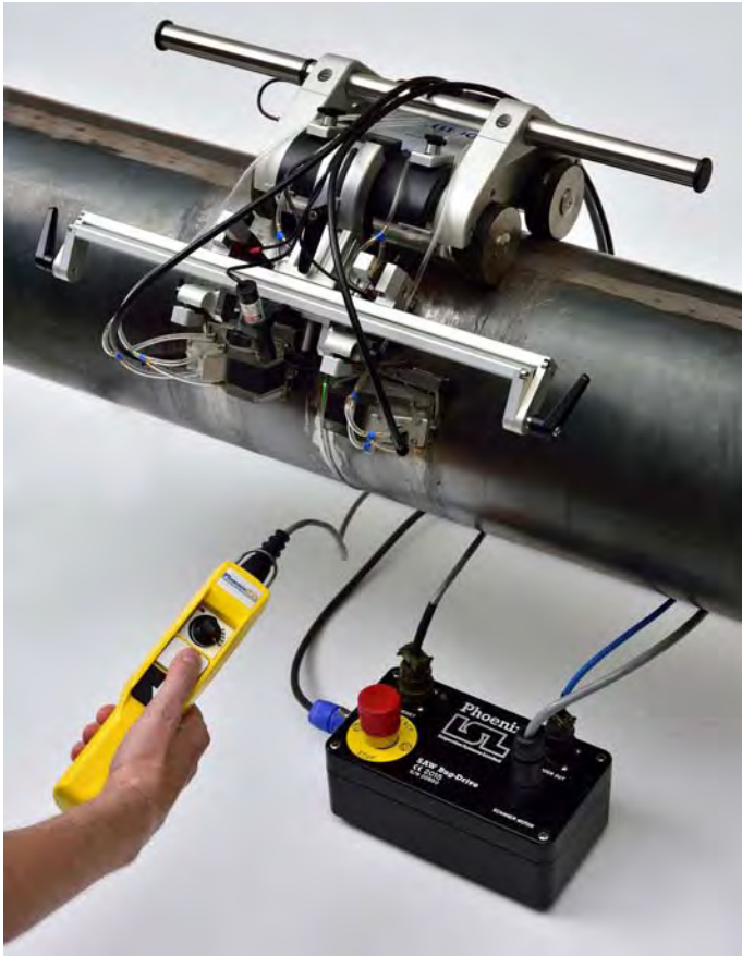
SAW Bug inspecting a 10"OD weld with TOFD and phased array probes
