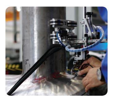
NozzleScan is a versatile, low-profile manual scanning solution developed for the inspection of nozzle welds in both setthrough and set-on configurations, with the option of a motorised version for automated inspection.
