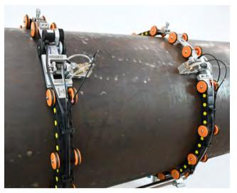
The Multi-Skip or M-Skip scanner offers an ultrasonic solution for corrosion detection of difficult to access areas of pipelines; around obstructions such as pipe supports, clamps and saddles.
