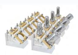
The adaptable scanner comprises of sets of interlocking belt sections that can be adjusted according to pipe diameter from 6" up to 48" OD (outside diameter). Separation bars ensure accurate and consistent probe and wedge placement around obstructions at distances of up to 1m (3.28ft).
