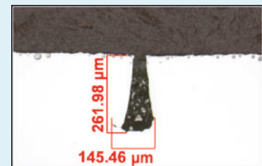
Cross section 2 Defect depth: 0.26 mm
