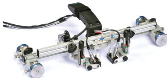
Dual direction Swift, with optional pivoting wheel units, for B scans with two TOFD probes
