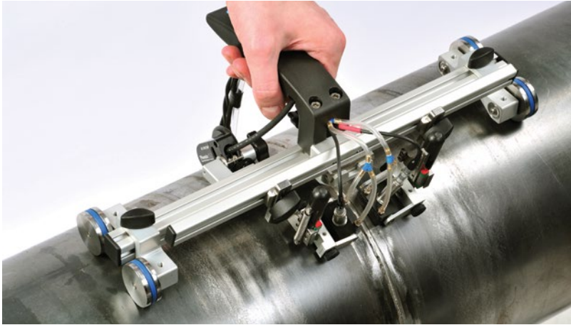
Single direction Swift configured for D scan of circumferential weld with two TOFD probes
